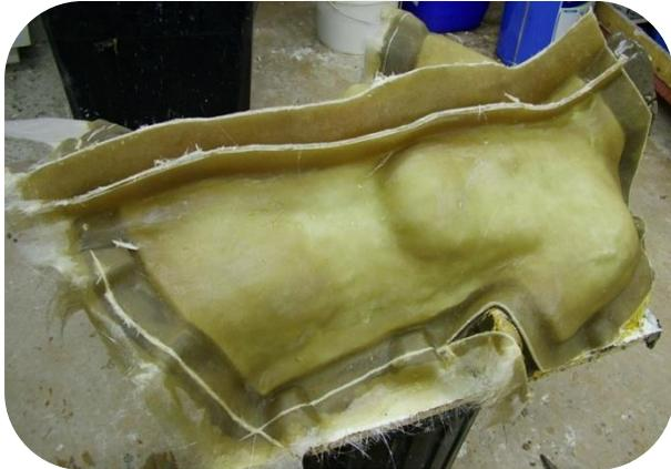
Fibreglass and polyester resin used to create a supporting jacket for a silicone mould. Mould by Stuart Bray for BBC TV's *Waking the Dead* (2008) for Waldo Mason.
